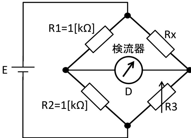
$$\begin{aligned} R_x &= \frac{R_1 R_3}{R_2} \\ &= \frac{1 \times 10^3 \times 2 \times 10^3}{1 \times 10^3} = 2 \times 10^3 \\ &= 2\text{[k}\Omega\text{]} \end{aligned}$$
