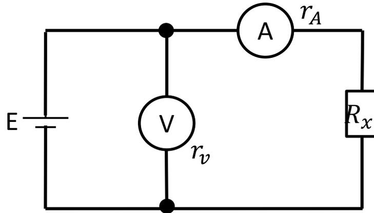
$$\text{式(2.8)} \quad R_x = \frac{V - r_A I}{I} \text{ より}$$
